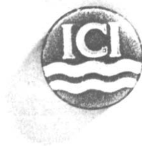
Fig. 1. A tablet previously coated with red iron oxide in hydroxypropyl methylcellulose further coated with the same film former containing calcium carbonate.
